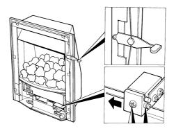
Unscrew the burner assembly fixing screws at either side of the firebox, and the two fixing screws at the base of the fire (See fig. 7 below).
