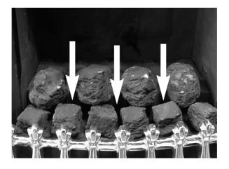
e) Select four of the medium coals and arrange along the rear of the fuelbed, using the recesses in the rear of the fuelbed as a guide for placement. (See fig. 17 below)
